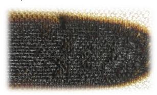
Microshield®s fiber impregnation protects the material by incorporating an intumescent solution into the fibers. When exposed to fire this foams and forms an effective fire protection layer.
